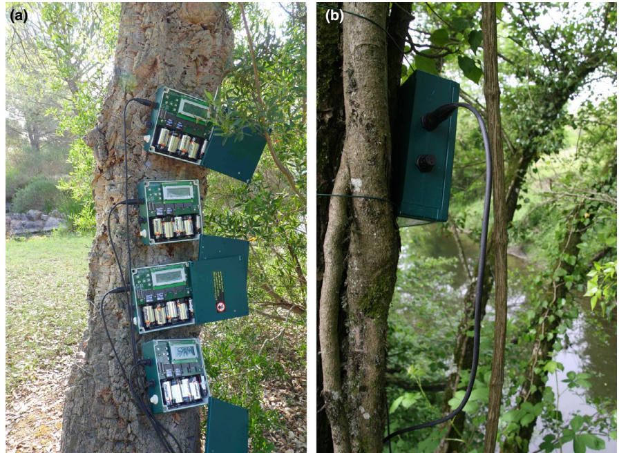
FIGURE 3 Pictures of typical recording set-ups. (a) Automatic recorders and hydrophones set up in a pond in Vidauban (France). (b) Automatic recorder set-up in a secondary channel of the river Rhône (France)
